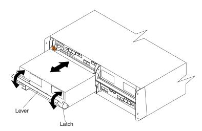
Figure 83. Replacing a power supply and fan unit
